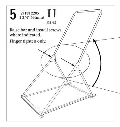
**Note:** Nuts should be installed on the outside of the floor stand.
