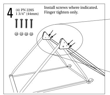
**Note:** Nuts should be installed on the outside of the floor stand.
