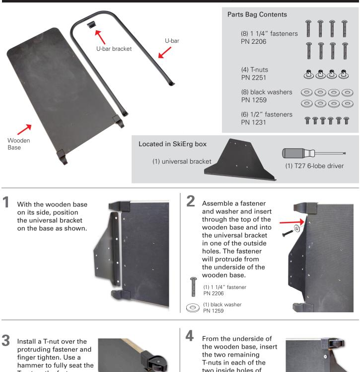
finger tighten. Use a hammer to fully seat the T-nut on the fastener. Repeat steps 2 and 3 on the opposite outside hole and tighten both fasteners.
