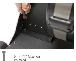
8 Using a fastener and washer, attach the U-bar to the wooden base on each side. Tighten until fully seated.
