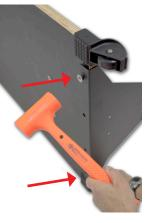
From the underside of the wooden base, insert the two remaining T-nuts in each of the two inside holes of the universal bracket. Use a hammer to fully seat the T-nuts. Lay the wooden base on its bottom in preparation for mounting the SkiErg.
